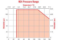
These graphs are intended to give you a general idea of the performance capabilities of each product line. The shaded area of each graph represents the operating range of the product family, i.e., upper and lower values are shown. Therefore, depending on the exact coupling configurations selected, you can reasonably expect values to fall within the shaded area.
