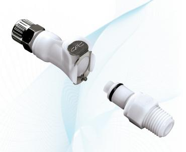
The 1/4" flow PLC Series is proven worldwide in thousands of applications and offers the widest selection of sizes and configurations. PLC couplings are injection molded from acetal thermoplastic and are resistant to most mild chemical solutions. One-hand connection/disconnection, plus integral terminations make the PLC Series the choice for ease of use and manufacture.
