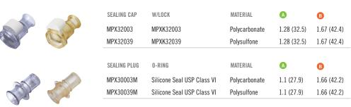
All measurements are in inches (millimeters) unless otherwise noted. Tubing must meet stated inside and outside diameters.
